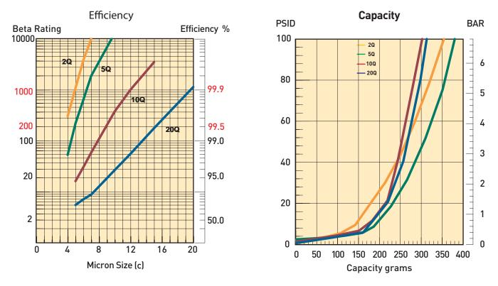
Results typical from Multi-pass tests run per test standard ISO 16889 @ 80 gpm to 100 psid terminal - 10 mg/L BUGL Refer to Appendix on pages 264-265 for relationship to test standard ISO 4572.
